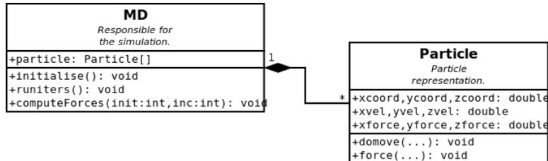
Fig. 2: Simplified MD class diagram.
